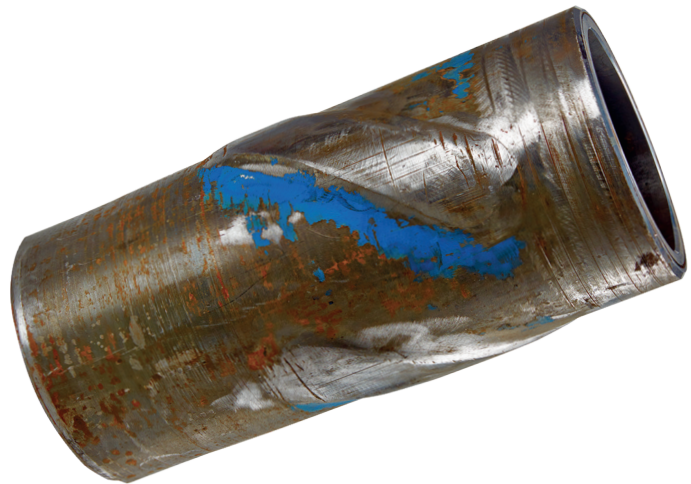
Figure 3. HydroFORM centraliser used in an extreme liner drilling application that required multiple trips. In this crimp-on application, the string had an accumulated running distance of 65 870 ft and over 41 000 revolutions, with the entire lot of installed centralisers remaining intact. Wear on the centraliser ribs measured less than ¼ in. on OD, or less than half of the original wall thickness.
