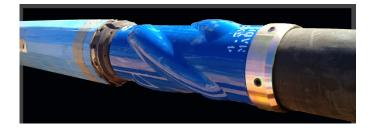
Volant's review of the measured surface loads during the successful run led the customer to consider more centralizers in the open hole section for future wells, reducing total friction. On subsequent wells, an additional centralizer was placed at each packer in the open hole section (one on each side of each packer), and the liner runs continued to be smooth with a substantial observed reduction in open hole friction factor of approximately 30%.
